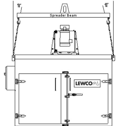
*Figure 1: Typical Rigging*
